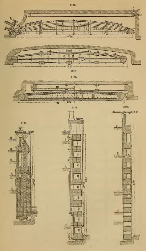
latter is formed of two pieces, the one on the down-stream side straight, the other curved and abutting upon it near the ends, the two being bound together by bolts, so as to constitute a single piece, having a thickness in the middle of 2 ft. 1 in.
